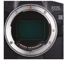
A 30.3 megapixel Full Frame Canon CMOS sensor delivers incredible image quality and detail from highlights and shadows
